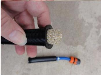
4. Cut a piece of shade-cloth about 30cm long by 2 cm wide and roll up. Push the rolled-up wad of shade cloth it into the open end of the inline filter insert to keep the fertiliser in place.
