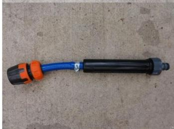
2. Add a short piece of hose (5-10cm is enough) to the outward end; then add a hose fitting to allow you to attach a water-breaker to the end. At the inward end, replace the screw-on fitting with a standard 1” tap fitting.
